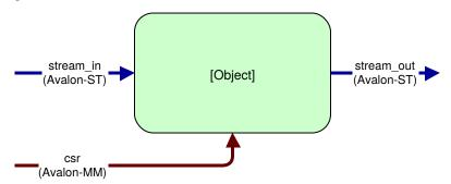
The DUT will swap the endianness of packets on the Avalon-ST bus if a configuration bit is set. For every packet arriving on the stream\_in interface the entire packet will be endian swapped if the configuration bit is set, otherwise the entire packet will pass through unmodified.
