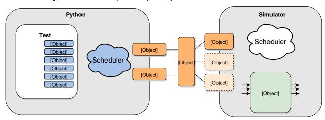
A test is simply a Python function. At any given time either the simulator is advancing time or the Python code is executing. The **yield** keyword is used to indicate when to pass control of execution back to the simulator. A test can spawn multiple coroutines, allowing for independent flows of execution.
